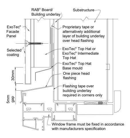
**Note:** When RAB® Board is used with timber frame flashing tape to be applied to the entire window opening
